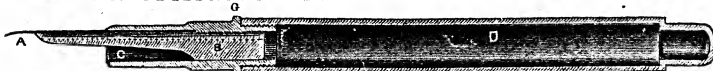
Sectional View. References—A, Gold Pen; B, Feed Bar; C, Point-section; D, Barrel; G, Knurl.
